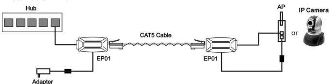
Note: The power voltage must go through a regulator (ref. page 2 optional model) if the output voltage is higher than the equipment voltage.
